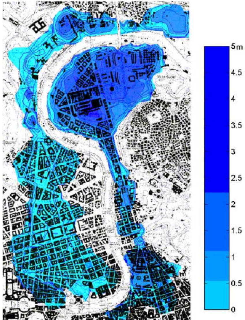
Figure 3 - Water depth distribution is shown after 24 hours from the beginning of the simulation.
