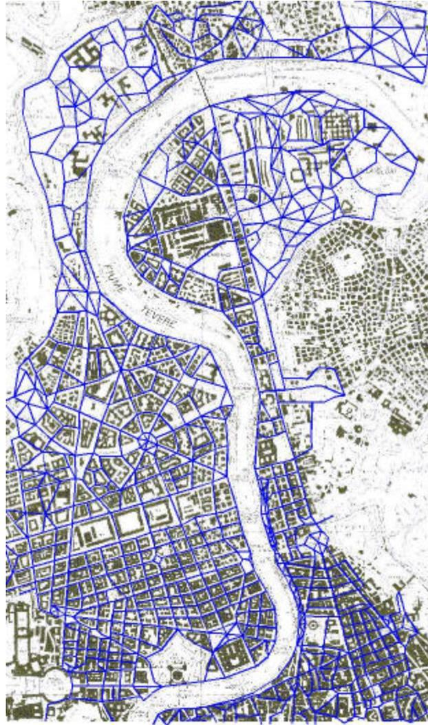
Figure 1 - The channel network used for the simulation
