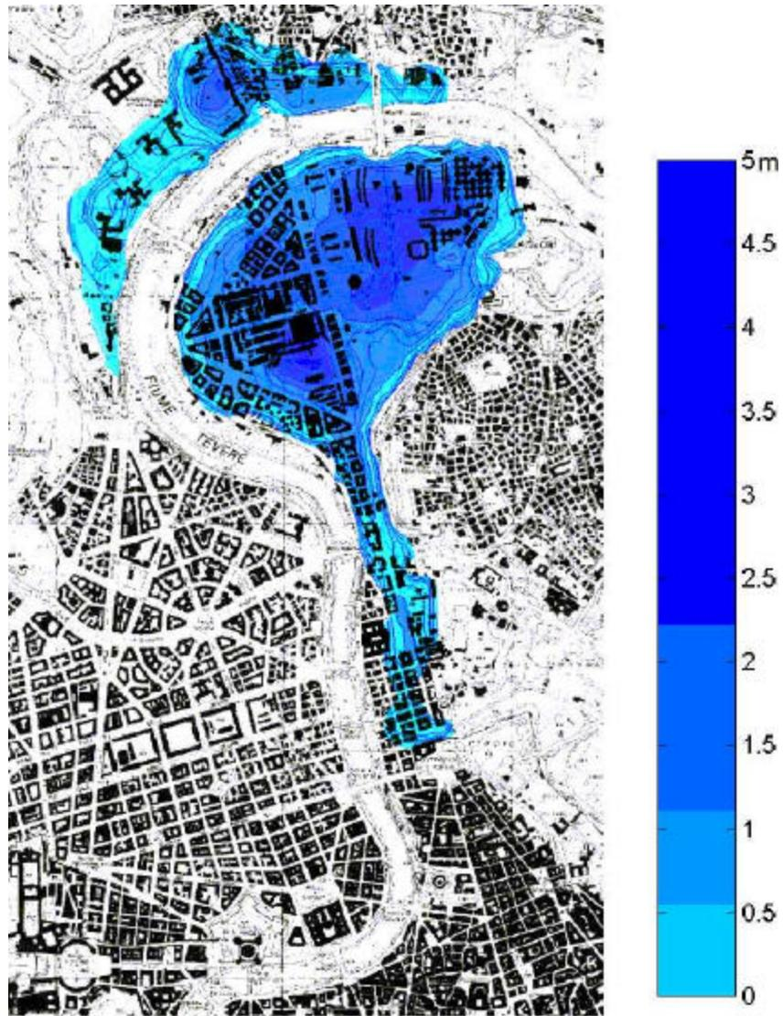
Figure 2 – Water depth distribution is shown after 6 hours from the beginning of the simulation.
